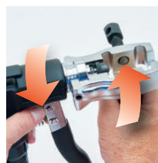
Two-piece design allows for swivel action
