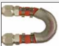
Rear Heater Core Block Off Repair
