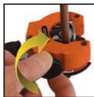
Spring-loaded automatic cutter. Snug down onto tubing, then turn knob 360°.
