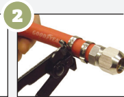
2 Crimp with clamp pliers
