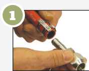
1 Place clamp onto hose, push adapter into hose
